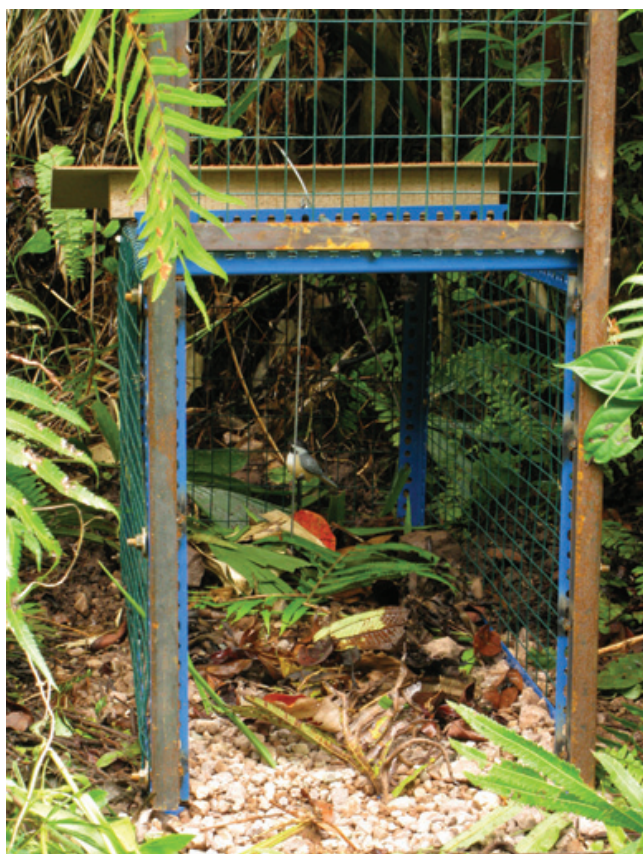
Fig. 4. Example of an electronic lure. A small box hidden in the vegetation at the bottom of the trap emits the sound of bird song and the plastic bird spins around when the sound plays. (Photograph by: J. Ross and A. J. Hearn).
