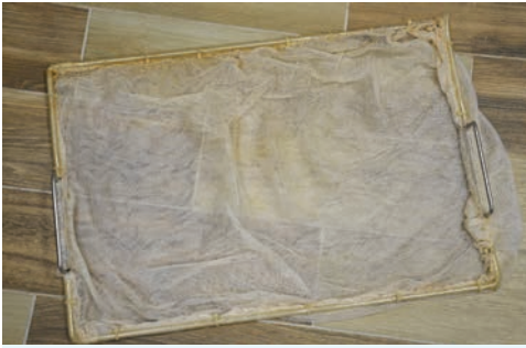
A 60 × 40 cm push net. This net is used to catch fishes and large macroinvertebrates
